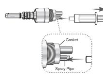
Cover the spray pipe with the end of a plastic disposable syringe with the needle removed. Press the end of the syringe flush against the gasket on the coupling so that it is air tight.
