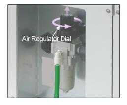
1. Pull up the dial on the air regulator and turn it until the pressure drops to 0 MPa.
