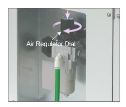
3. After draining the regulator, turn the dial back to adjust the pressure and push it back down.
