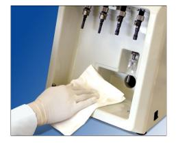
4. Clean the main body with a neutral detergent or Ethanol for Disinfection (Ethanol 70 vol% to 80 vol%).
