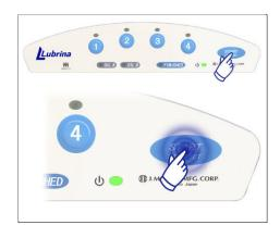
4. Check the time setting by how fast the lamp blinks, and then press the Start Switch for 2 seconds.
